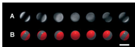
Figure 4. 3D analysis of patterned membranes in different view angles with digital video microscopy. A) Fluorescence time-lapse images of membrane patterns on a single 7 μm colloidal-silica particle lying on the substrate. B) Simulated images in each corresponding angle of view. Membranes are seen to be nicely patterned three-dimensionally throughout the colloidal surface, and membrane patterns are in good agreement with simulations. The bar represents 7 μm. Membrane composition: 99% DPPC and 1% Texas Red DPPE.
